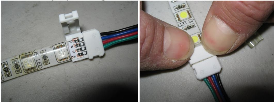
8. This connector will hold the ribbon and make a solid electrical connection as well. Check to be sure the ribbon is tightly secured by **gently** tugging it to make sure it doesn't pull out easily & LEDs still light.
