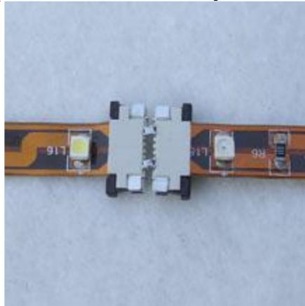
10. Here's the connected 2-wire ribbon-to-cable connector:
