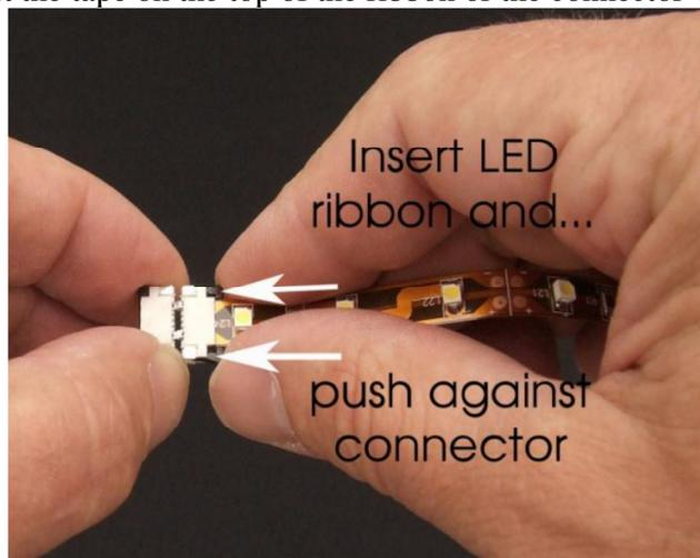
8. This connector will hold the ribbon and make a solid electrical connection as well. Note the position of the black slider, which has been pushed to the left into the white piece.
