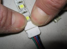
8. This connector will hold the ribbon and make a solid electrical connection as well. Check to be sure the ribbon is tightly secured by **gently** tugging it to make sure it doesn't pull out easily & LEDs still light.
