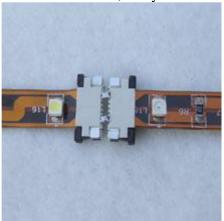
10. Here's the connected 2-wire ribbon-to-cable connector:
