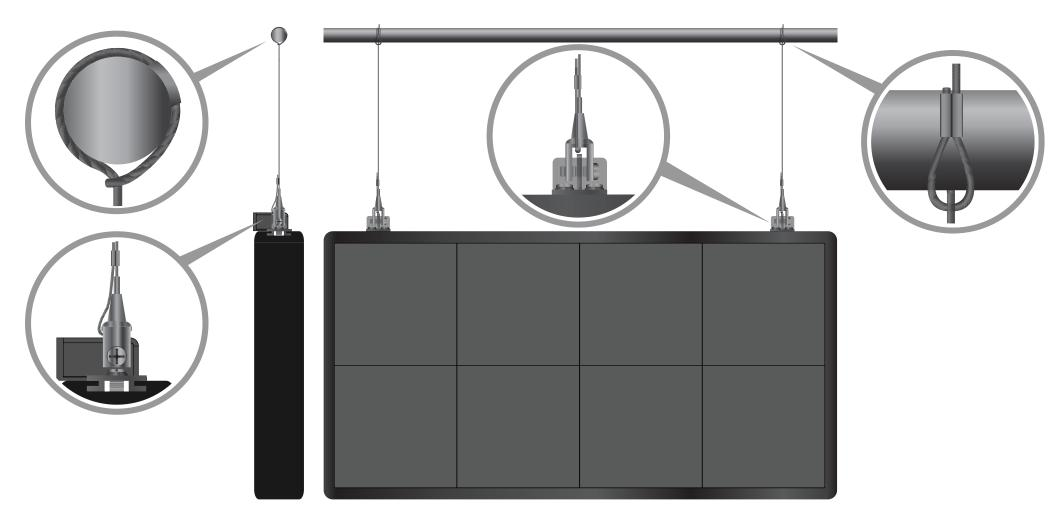
CAUTION DO NOT weld any part of the MLS cabinet or the General Bracket; Bolt General Bracket and MLS cabinet ONLY! DO NOT drill additional holes into either the General Bracket or the MLS cabinet. DO NOT house the MLS inside other enclosures. These actions, including but not limited to, VOID all warranties. (Note: Again, it is very important that your check with local building and planning department for codes and laws regarding signs and their installation.)
